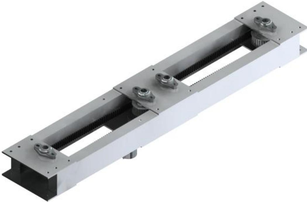
**Figure 10: "Steering Pod" Design**
