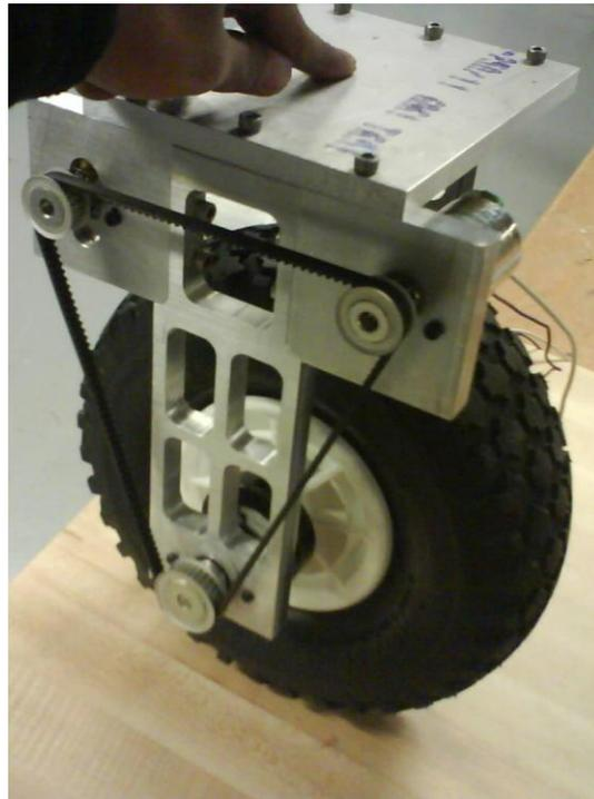
**Figure: Fabricated DrivePod. Initial Version**
