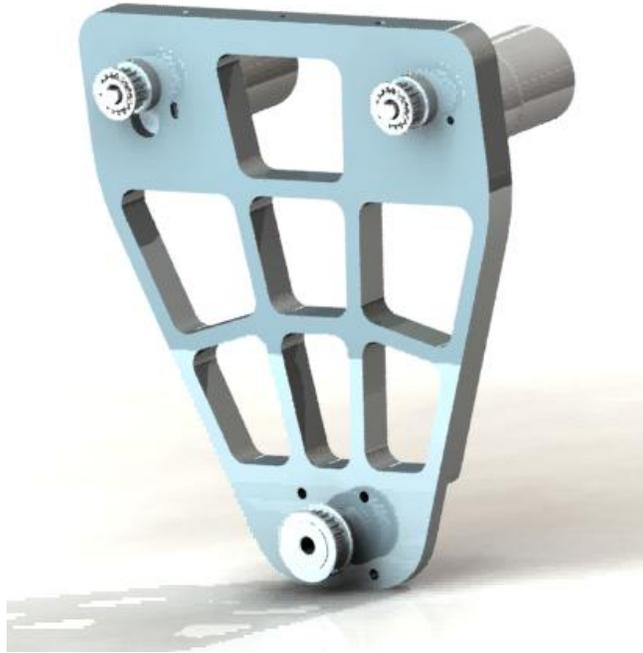
**Figure 4.2: V Plate Rendering with attached Motors and Pulleys**
