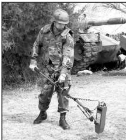
Figure 1: Nomadics Inc.'s fluorescent detector
